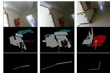
Fig. 10. Processed successive frames, the planes located in 3D: ground for the third frame (red color), ceiling (blue color in the first two frames ), walls (white color), projected wall on the floor plane. The inner angle for this case is equal to  $270^\circ$ .
