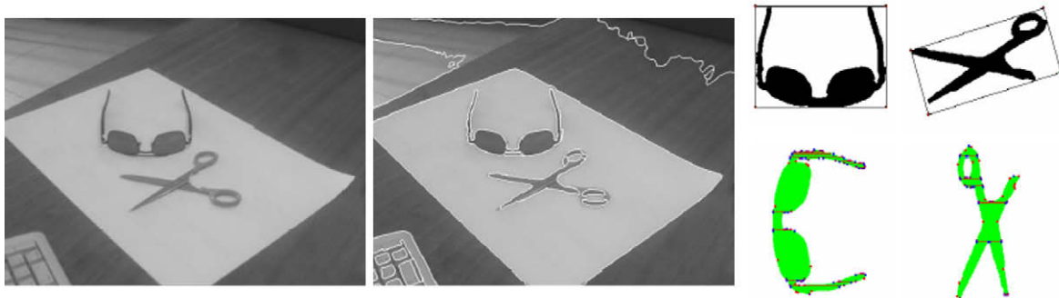
Fig. 27. Different steps applied for the computation of XLWDS descriptors for the two extracted silhouettes (glasses and scissors).
