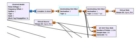
Give it an identifier: lp for example, then add a Decimating FIR Filter block by typing in tps: lp
