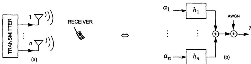
Fig. 11-7. (a) A wireless link with transmit diversity; (b) its equivalent narrowband model.
