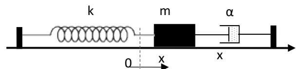
$$\frac{d}{dt} \left( \frac{\partial L}{\partial \dot{x}} \right) - \frac{\partial L}{\partial x} = - \frac{\partial D}{\partial \dot{x}}$$
