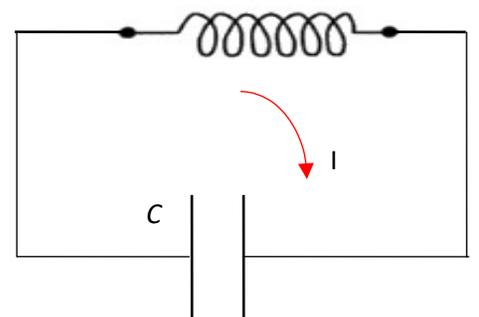
$$V_L = L \frac{dI}{dt}, V_c = \frac{q}{C} \text{ comme } I = \frac{dq}{dt} = C \frac{dV_c}{dt}$$
