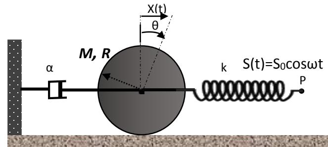
On donne  $s_0 = 10\text{cm}$ ,  $\omega = 10 \text{ rad/s}$ ,  $M = 1\text{kg}$ ,  $\alpha = 60 \text{ kg/s}$
