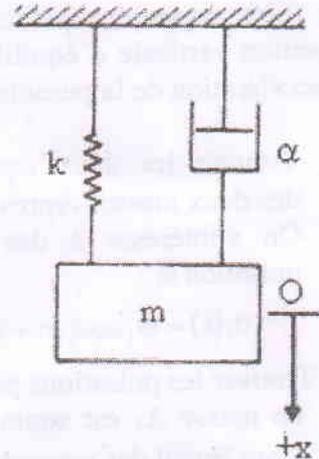
$$x(t) = e^{-\delta t} \left\{ x_0 \cos \sqrt{\omega_0^2 - \delta^2} t + \frac{\dot{x}_0 + \delta x_0}{\sqrt{\omega_0^2 - \delta^2}} \sin \sqrt{\omega_0^2 - \delta^2} t \right\}$$
