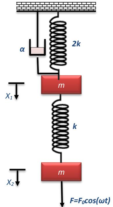
$$z_1 = \frac{\begin{vmatrix} 0 & -\omega_0^2 \\ F & (\omega_0^2 - \omega^2) \end{vmatrix}}{\begin{vmatrix} (3\omega_0^2 - \omega^2 + \frac{i\alpha}{m}) & -\omega_0^2 \\ -\omega_0^2 & (\omega_0^2 - \omega^2) \end{vmatrix}} = \frac{\omega_0^2 F_0 e^{i\omega t}}{(3\omega_0^2 - \omega^2 + \frac{i\alpha}{m})(\omega_0^2 - \omega^2) - \omega_0^4}$$
