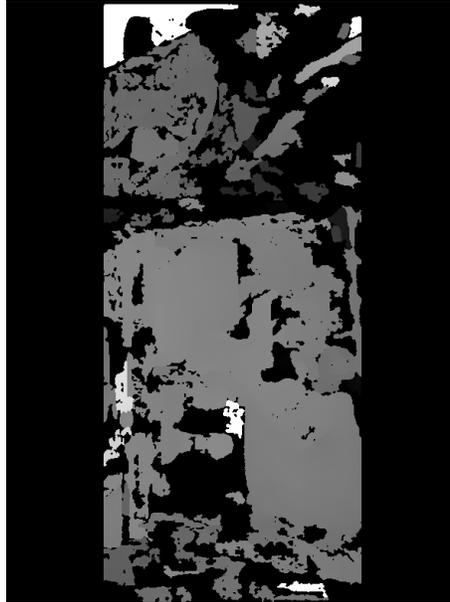
**Fig. 1.5** The computed depths using the rectified images based on the horizontal disparity of matched points .
