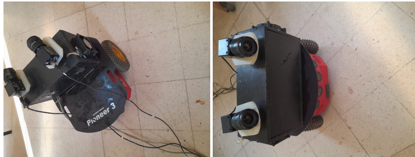
Fig. 1.2 A Pioneer 3DX, embedded with a stereoscopic system.
