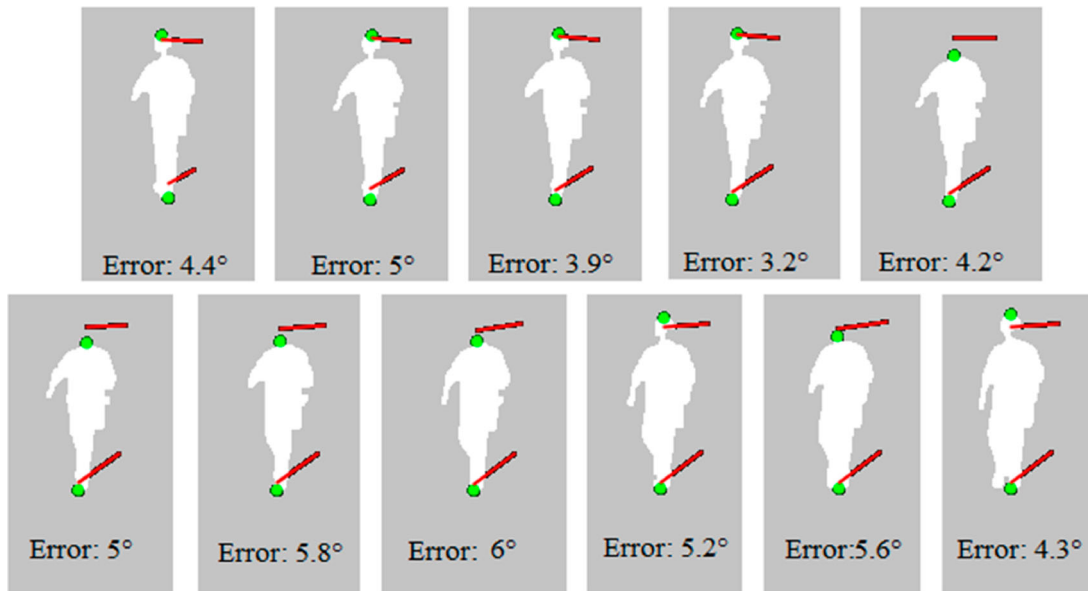
Figure 12. Direction computation of walking pedestrian for successive frames of Casia-B dataset (Ground truth direction: 18°). Note that despite the missing of head in some frames, the error of estimated direction remains stable (5°).
