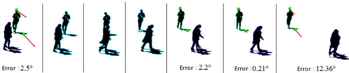
Figure 14. Example of failure when groups of pedestrians are walking in different directions are grouped (case of second, third and fourth frame).
