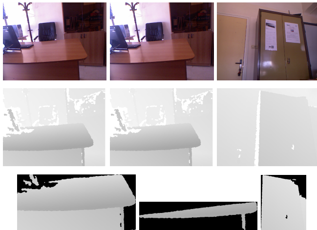
Fig. 16 From top to down: the captured scene (table, table, dresser), its associated depth image (the system input), the resulting segment. The system has predicted: table, chair and dresser.
