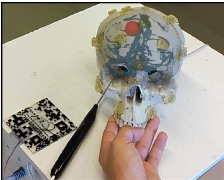
Figure 4. An AR view of a projected skull using the HoloLens 2 and a multimodal marker.
