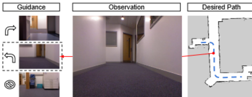
Figure 2.2: An example of indoor mapless based Navigation system with sparse directional guidance. The robot automatically selects from the provided guidance based on current observation. Source: [14]
