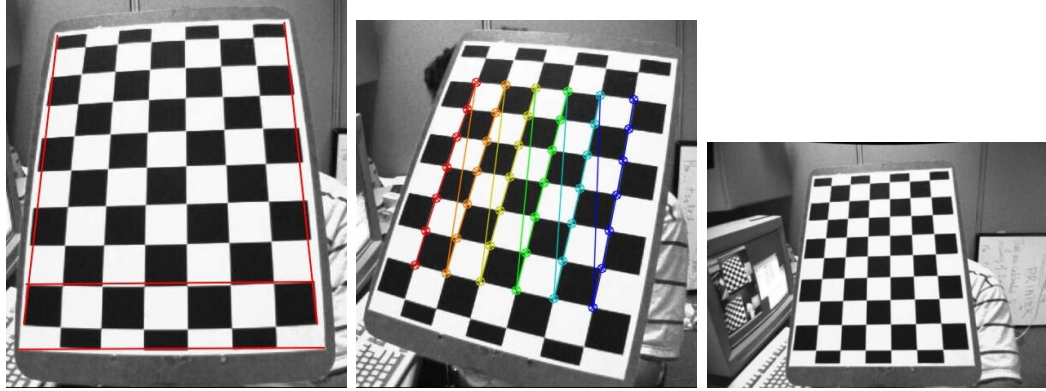
Figure 3.4: Camera calibration [9]. From left to right: an image with distortion, the chess-board pattern used to compute the distortion parameters, and the image results after calibration (the distortion is eliminated: the edges are straight).
