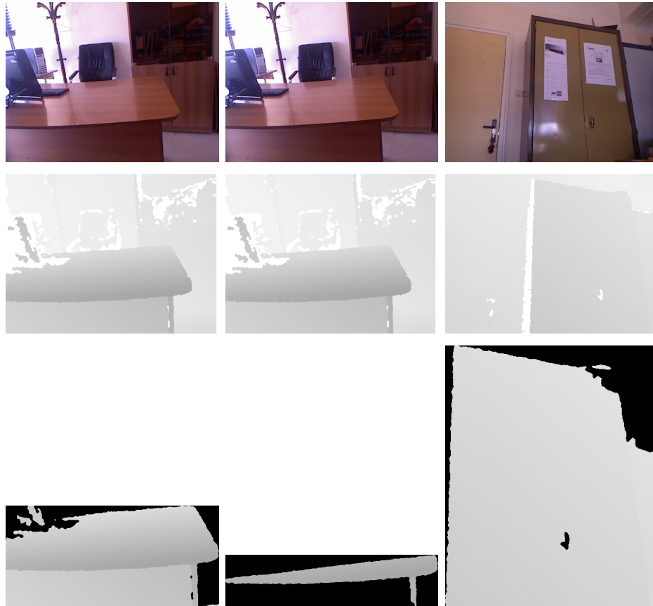
Figure 5.27: From top to down: the captured scene (table, table, dresser), its associated depth image (the system input), the resulting segment. The system has predicted: table, chair and dresser.
