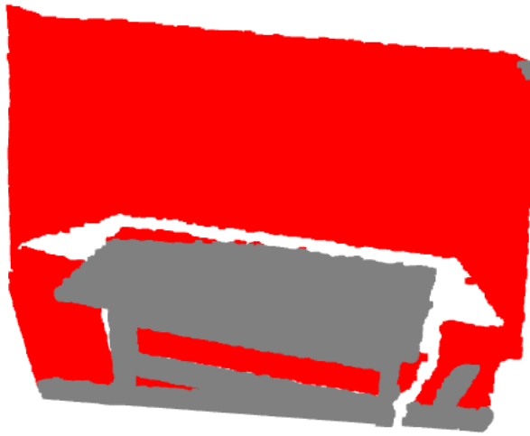
Figure 3.7: Pass-through filter. The red points will be neglected since they are out of the fixed interval [1500, 2000]mm .
