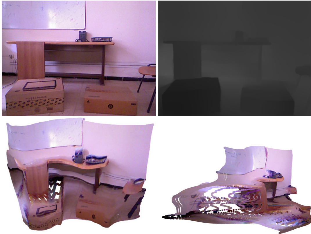
Figure 3.6: Point cloud estimation using DenseDepth neural network. First row: the input image (left) and the generated depth map (right). Second row: two views of the generated point cloud. The depth image is over smooth; thus, the point cloud is distorted.
