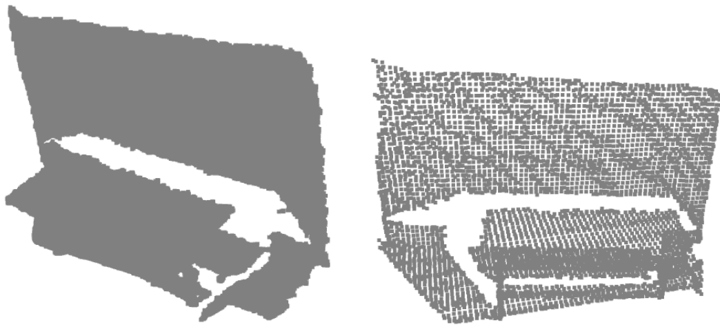
Figure 3.8: Left: the point cloud. Right: the point cloud after voxelization (in this example, we took l = 5mm ). The point cloud is smoothed and its size has been reduced.
