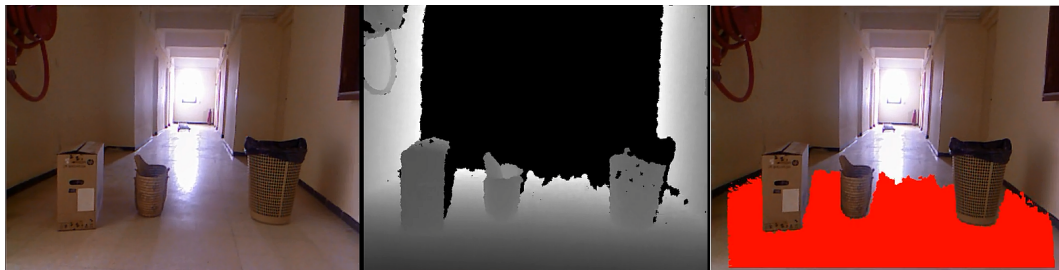
Figure 4.20: From left to right: Color image, depth image, ground colored with red color.
