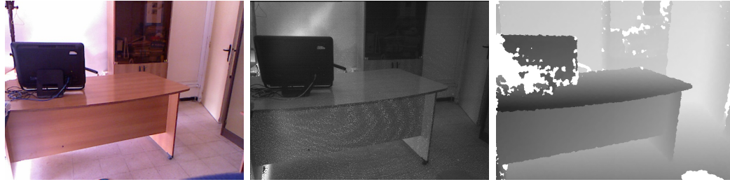
Figure 3.3: Microsoft Kinect's produced data. From left: RGB image, IR image and Depth image.
