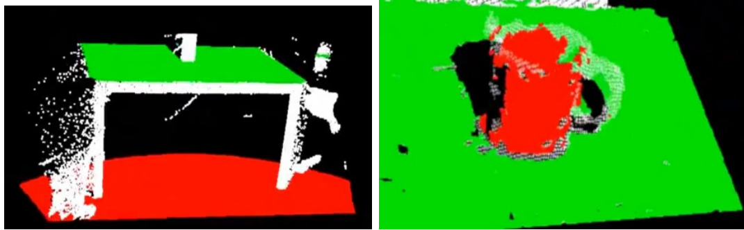
Figure 3.12: RANSAC for segmentation [10]. Green color and red color respectively represent the detected plane and cylinder.
