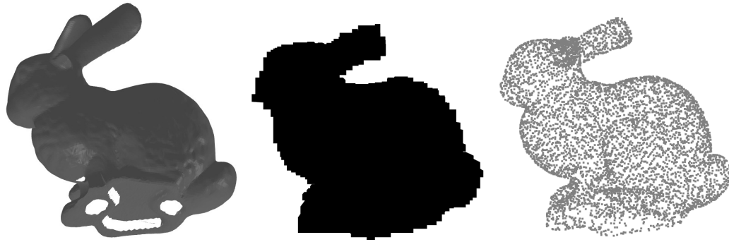
Figure 3.14: Stanford bunny. From left to right: a single 2D view representation, volumetric representation and point cloud raw representation.
