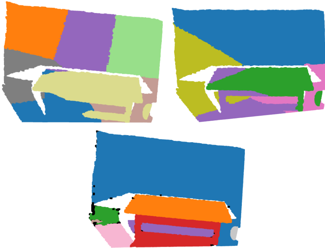
Figure 3.13: Point cloud clustering: k-means (top left), mean-shift (top right) and DBSCAN clustering (bottom). We first applied DBSCAN algorithm; it returned K clusters ( K = 7 ) that is used to set the number of the clusters for k-means and mean-shift algorithms.
