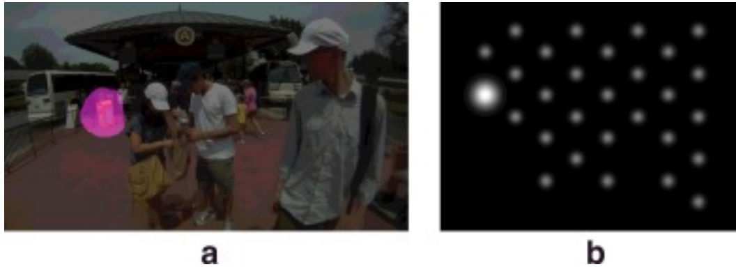
Figure 2.1: Horne et al. [4]: (left) the task of finding the garbage. (right) the produced semantic labeling: the garbage is represented with high-intensity phosphenes and the obstacles with low-intensity phosphenes. The user can follow the gaps to the target.
