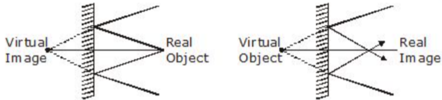
Figure: Object space and image space for a plane mirror - symmetric configuration
